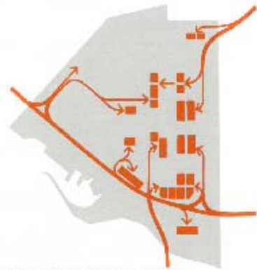
Expressways Feed Into Parking Structures
